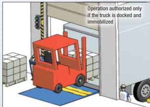
First pallets position : The onstacle retracts at the same time the refuge fills and allows the truck to take the first pallets at the end of the trailer.
