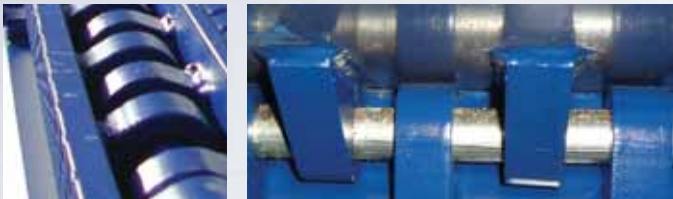
Highly resistant oxy-cut lip hinges in the form of drops of water: The more the capacity is high, the more the number of hinges is high.
