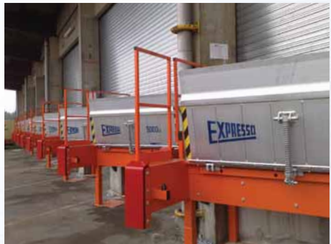
8860 ramp with sliding bumpers BUM0115 and serrated grating floor
