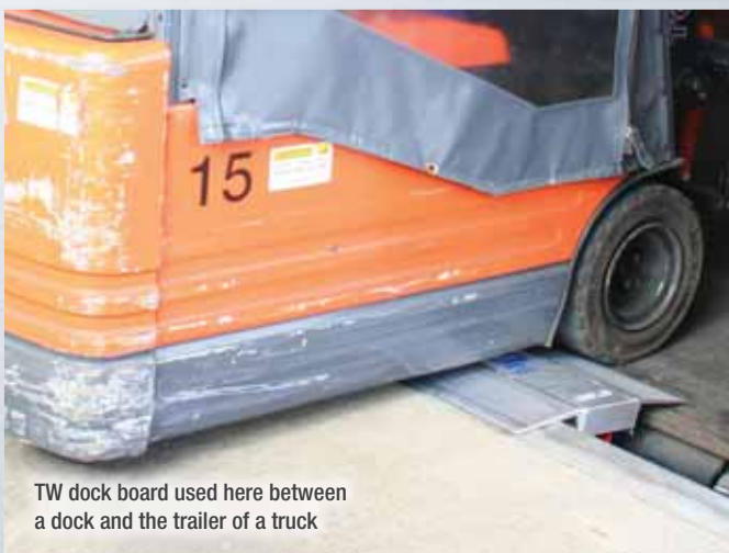
TW dock board used here between a dock and a wagon
