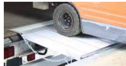
Forklift truck (Maximum load 6000 kg - Maximum slope 10%*)
