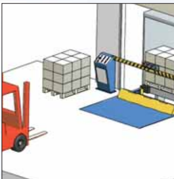
The truck is docked, the door is open but a pallet placed at the end of the trailer prevents full deployment of the leveler ...
