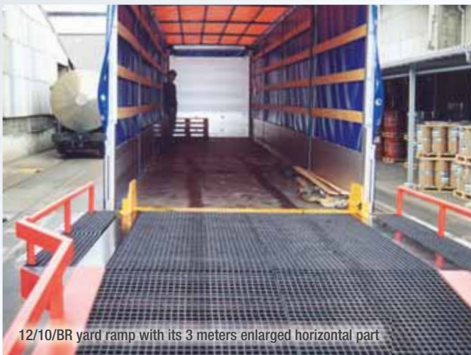
12/10/BR yard ramp with removable side crash barriers
